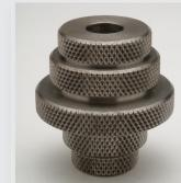
Knurling is a thread rolling process that produces a raised diameter on a part. It allows for a better grip compared to a smooth metal finished part. Knurling is also utilized to create a pressed fit into a controlled diameter. Additionally knurling is used to raise a worn diameter, as needed.
